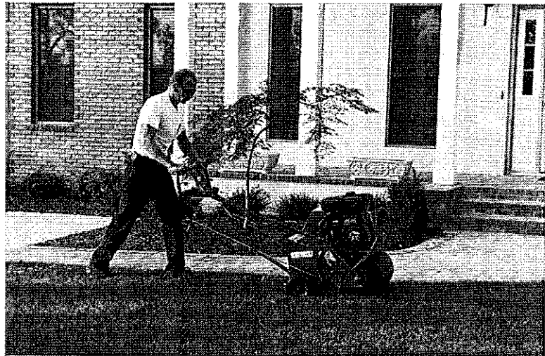
FIGURE 3. A self-propelled aerator is being used to promote turf growth.
